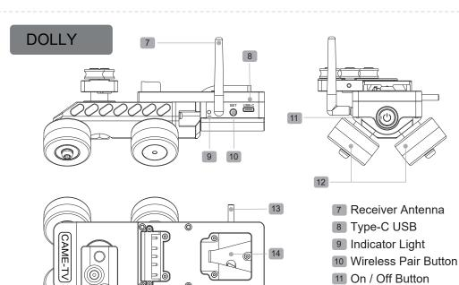
12 Power Drive Wheel13 V-mount Battery Lock
