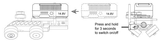
Important: Please correctly select the 12V--16.8V V mount Battery for photography to supply power to the device, otherwise it is easy to cause bad or serious consequences!
