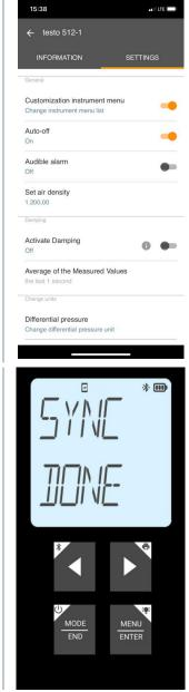
Changes to the measuring instrument settings in the app are transferred directly to the measuring instrument. Synchronization with the app is confirmed on the measuring instrument via "SYNC DONE".
