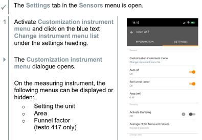
Temperature Change temperature unit Air velocity Change unit 2 Deactivate the checkboxes for the measuring instrument menus that are no longer to be displayed on the measuring instrument itself.
