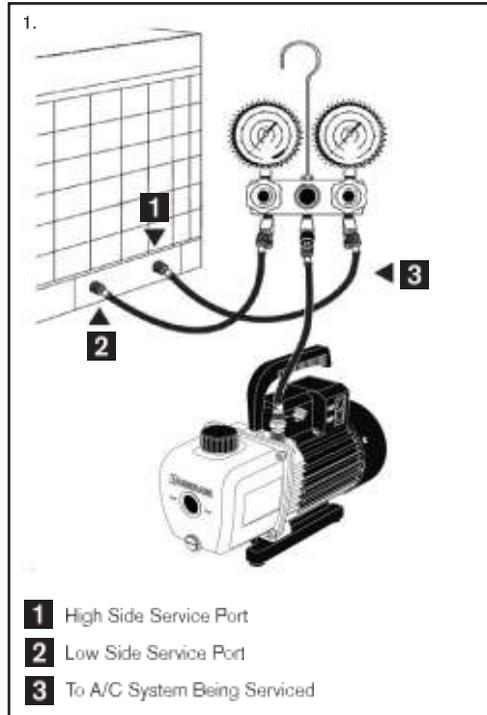
3. Open all manifold valves and system service valves, if applicable.
