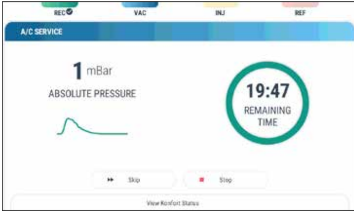
«Vacuum» phase: a vacuum is induced in the vehicle's A/C system to check for possible leaks.
