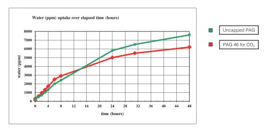
While the water absorbed by the PAG is not free (but linked to PAG) and does not cause problems that may be associated with the free moisture, the reduced hygroscopicity exhibited by PAG 46 for  $CO_2$  can be obtained through a careful choice of the end-capped hydroxyl. A maximum water content (0.05%) has been defined for PAG 46 for  $CO_2$ .
