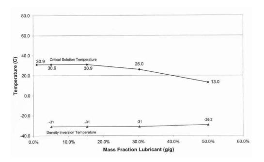
Even the upper critical temperature remains constant over a wide range of lubricant concentrations. The lower critical temperature does not occur, even if an inversion of density in the liquid phases is observed in the tested range of concentration.
