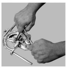
Turn handle clockwise until desired degree of bend is obtained. Handle may be extended to full width to give maximum leverage. To remove bent tubing pull out center pin, thus releasing forming wheel
