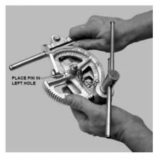
Attach forming wheel with hook point facing down and chained center pin inserted in left hole. Bender body handle will be closest to you and shoe, farthest away. Drop hook in place over tubing.
