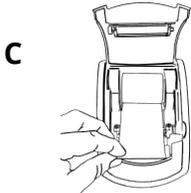
3. Pull a piece of the paper out through the feeder and then close the top cover. Figure C.
