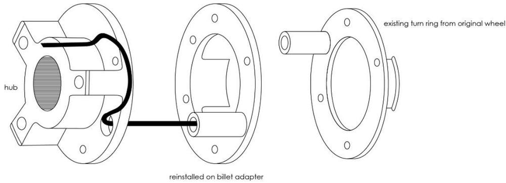
1. Remove turn signal cam from original steering wheel.
