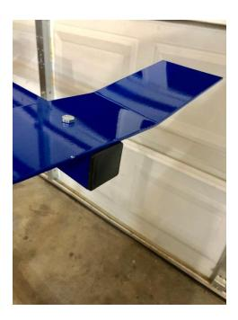
Locate and Install the (2) cradle platforms using (2)  $\frac{1}{2}$ " bolts with nuts. After the platforms are mounted, install the end caps using a rubber mallet.
