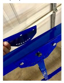
Locate and install top pivot bar using the (2) side plates, 3/16 Alan shoulder pivot bold with nut and (2) ½" bolts with nuts. Securely tighten and install pivot ball push pin.
