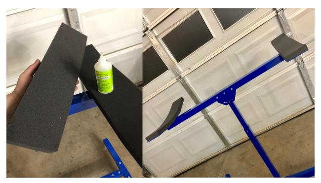
Use medium CA around the edges and center of the foam and locate the foam onto the cradle platforms. Keep pressure on them until the CA sets.
