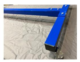
Install end caps on all 4 corners using a rubber mallet.
