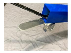
NOTE: after assembly lube the wheel bearings with WD-40 or equivalent to help spin freely.
