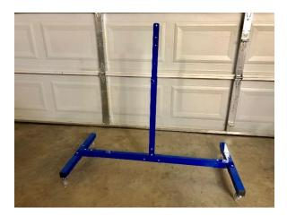
Slid adjustable center tube into place and install ball push pin.
