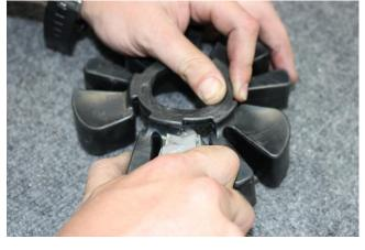
**2B** Place rubber cush upside down and cut away molding from all 5 cush sections as shown above using a utility knife.
