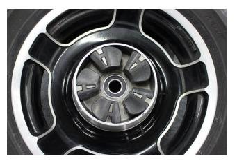
**2D** Reinstall the 5 individual cush drive sections back onto the wheel as shown above. Proceed to step 3
