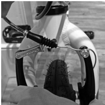
✘ This is not connected
