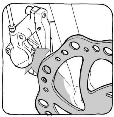
The ROTOR should slide inbtween the pads of the brake, easily.
