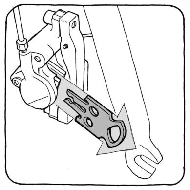
Spacer will come fully inserted into the front brake body between the pads to keep them from closing on eachother. Remove right before inserting installing front wheel.
