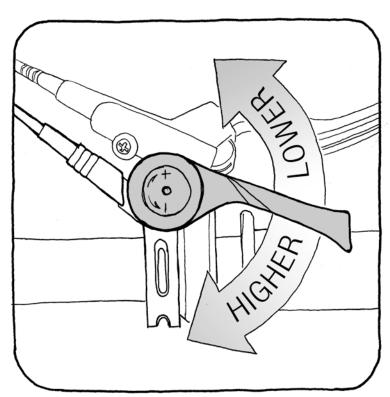
Thumb lever forward to shift to a lower gear.
