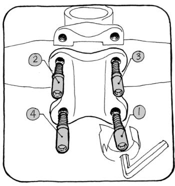
Working in an "x" pattern, tighten each of the bolts about 1/4 turn per pass to keep the tension even.
