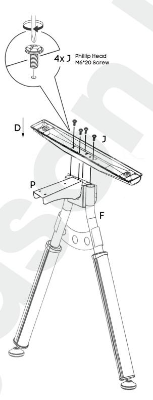
Note: Top Plate should lock Cantilever Bracket (P) into place
