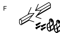
F Wardrobe Hanging Rod-2 PCS Wardrobe Hanging Rod Holder -4 PCS CSK Tapping Screw #8 x 3/8"- 8PCS
