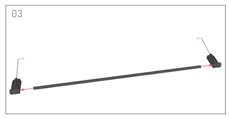
Fit the pullbar into the side-handles.
