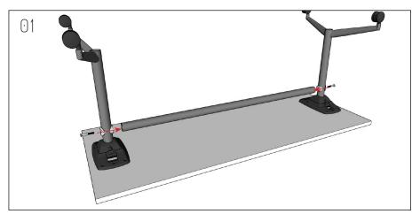
Place the drop-rail cross tube (45mm diameter) between the legs and fully tighten the M8x80 bolts through the plugs into the drop-rail. Making sure the notch in the end of the drop-rail cross tube is in-line with the bumps on the frames.
