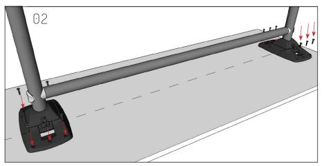
Pencil mark the centre-line of table top underside. Locate the frame in the centre of worksurface and fully tigthen using the M5x30 screws.
