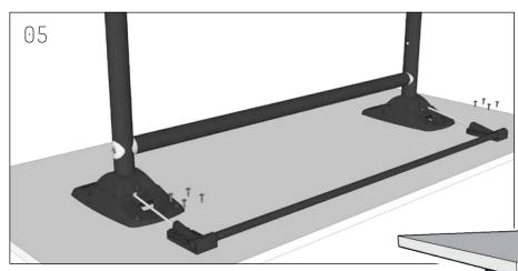
Screw fix the side-handles using M5x30 wood screws.
