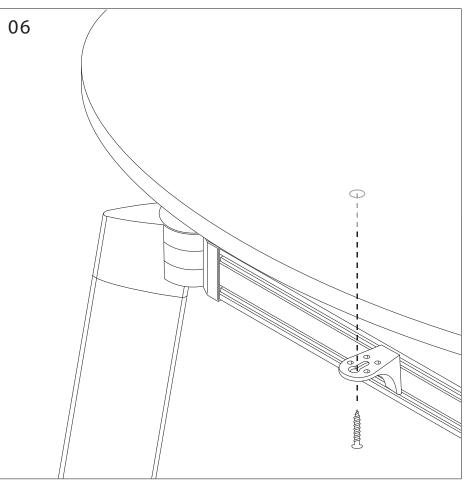
Directly screw into table tops, using L-Bracket screws through each L-Bracket.
