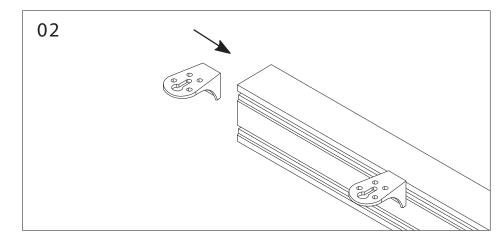
Join 1 L-Bracket through each Switch Beam
