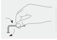
If this bolt does not drop into the joint use the Allen key to screw it all the way in so that it creates its own thread. This will ensure a nice, tight joint. **Note:** It is important to fully tighten all bolts and screws before attaching the top(s) so that the frame is sufficiently rigid. Failure to do this may affect stability once the tops are attached.
