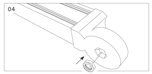
Insert Hex Nut on each Beam Bracket.
