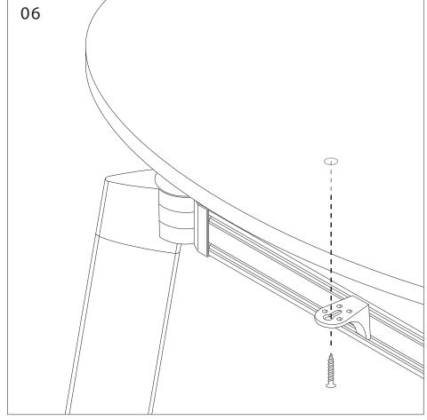
Directly screw into table tops, using L-Bracket screws through each L-Bracket.
