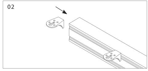
Join 1 L-Bracket through each Switch Beam
