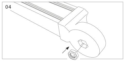
Insert Hex Nut on each Beam Bracket.
