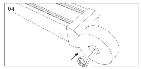
Insert Hex Nut on each Beam Bracket.
