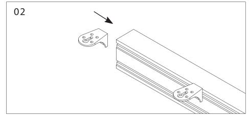
Join 2 L-Bracket through each 580mm Beam and 2 L-Bracket through each 1440mm Beam
