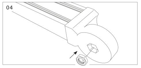
Insert Hex Nut on each Beam Bracket.
