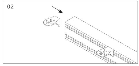
Join 2 L-Bracket through each Long Beam and 2 L-Bracket through each Short Beam.
