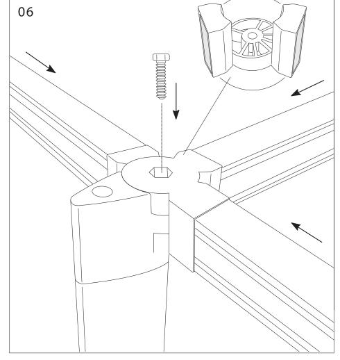
For the T central leg, attach as presented, using T Beam Bracket.
