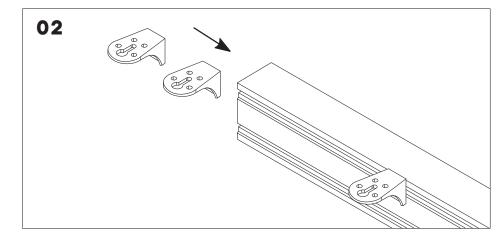
Join 3 L-Bracket through each Long Beam and 2 L-Bracket through each Short Beam.
