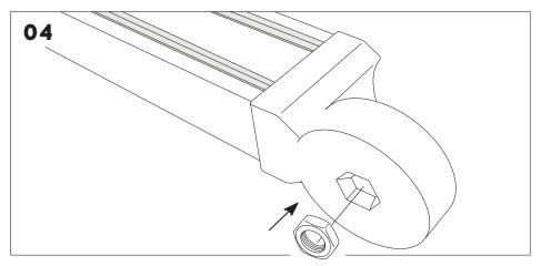
Insert Hex Nut on each Beam Bracket.
