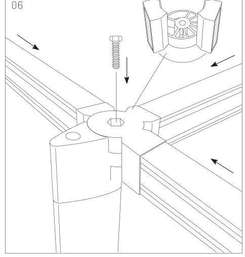
For the 4 central legs, attach as presented, using T Beam Bracket.
