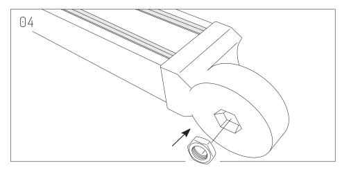
Insert Hex Nut on each Beam Bracket.
