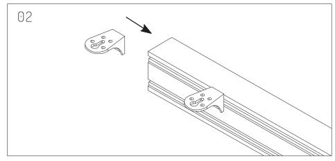
Join 1 L-Bracket through each Beam.
