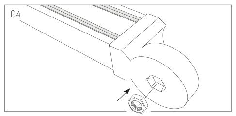
Insert Hex Nut on each Beam Bracket.
