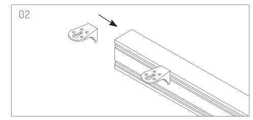
Join 1 L-Bracket through each Beam.
