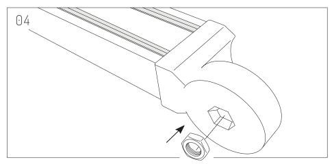
Insert Hex Nut on each Beam Bracket.
