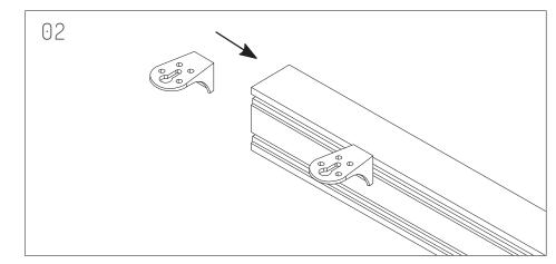
Join 1 L-Bracket through each Beam.
