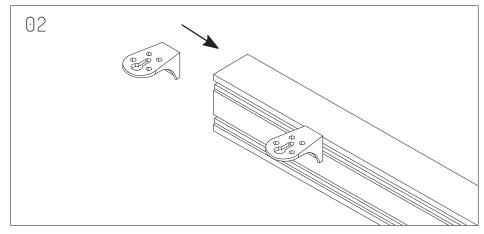
Join 1 L-Bracket through each Beam.
