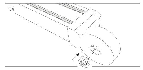
Insert Hex Nut on each Beam Bracket.
