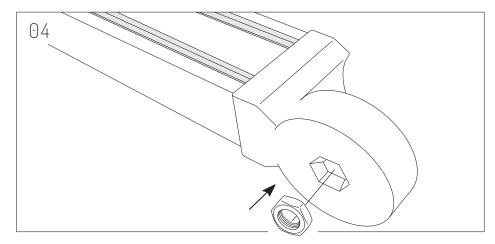
Insert Hex Nut on each Beam Bracket.
