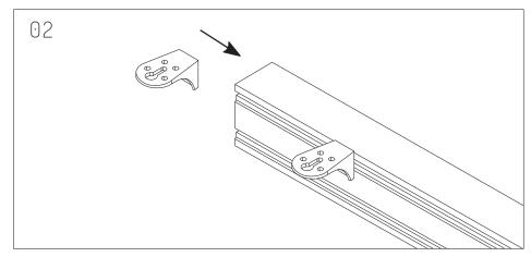
Join 1 L-Bracket through each Beam.
