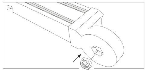
Insert Hex Nut on each Beam Bracket.
