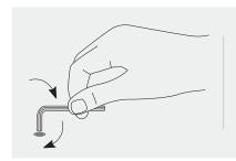
If this bolt does not drop into the joint use the Allen key to screw it all the way in so that it creates its own thread. This will ensure a nice, tight joint.
