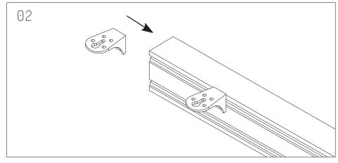
Join 1 L-Bracket through each 1515mm Beam and 1 L-Bracket through each 225mm Beam.
