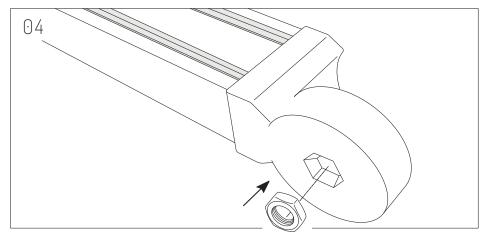
Insert Hex Nut on each Beam Bracket.
