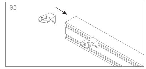
Join 1 L-Bracket through each 1315mm Beam and 1 L-Bracket through each 225mm Beam.
