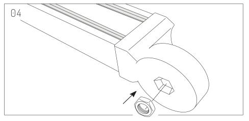
Insert Hex Nut on each Beam Bracket.
