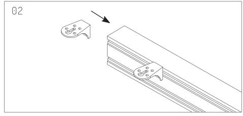
Join 1 L-Bracket through each 1115mm Beam and 1 L-Bracket through each 325mm Beam.
