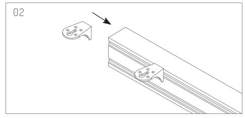
Join 1 L-Bracket through each 1115mm Beam and 1 L-Bracket through each 225mm Beam.
