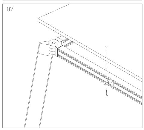
Directly screw into table tops, using L-Bracket screws through each L-Bracket.
