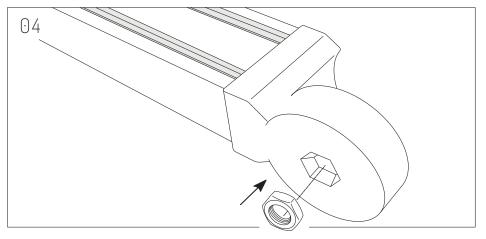
Insert Hex Nut on each Beam Bracket.
