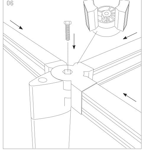
For the 2 central legs, attach as presented, using T Beam Bracket.
