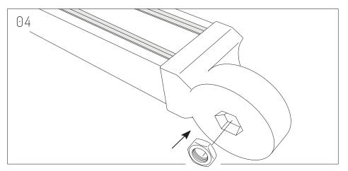
Insert Hex Nut on each Beam Bracket.
