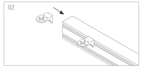
Join 1 L-Bracket through each 1315mm Beam and 1 L-Bracket through each 325mm Beam.
