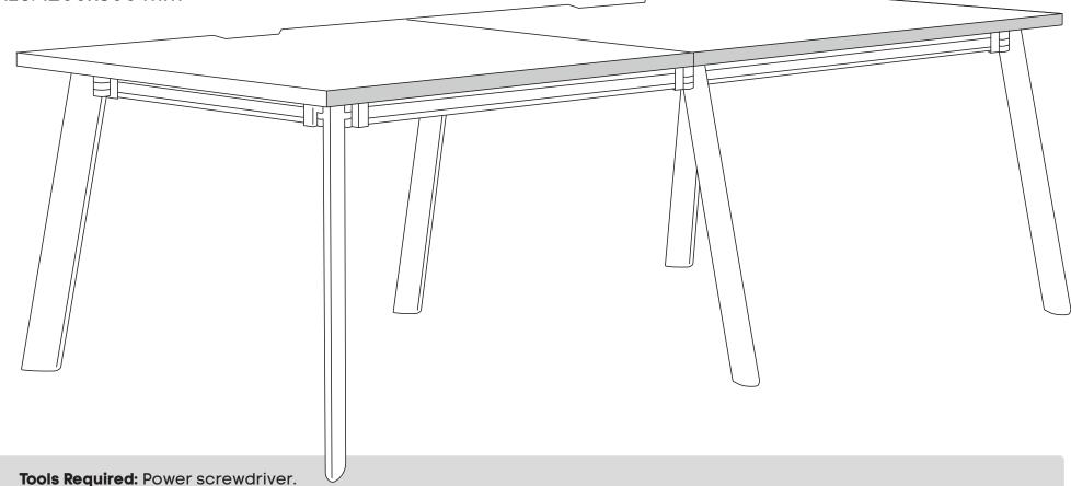
**Note:** Please ignore any pre-drilled holes or nut inserts that maybe present in your top(s). They will not match your particular table/desk base and woods screws will be required to be screwed directly into the underside of the top.
