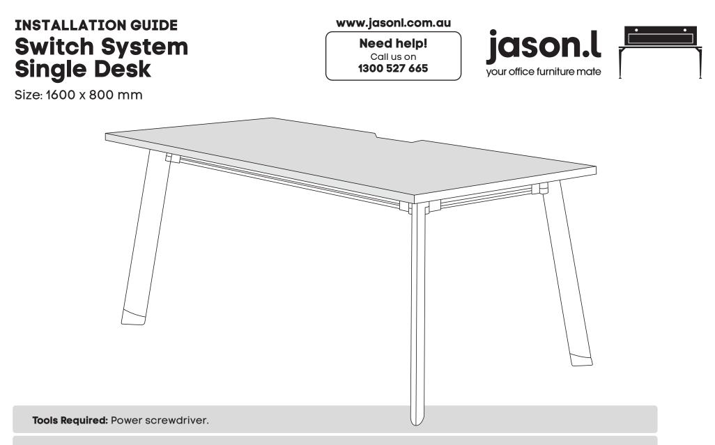
**Note:** Please ignore any pre-drilled holes or nut inserts that maybe present in your top(s). They will not match your particular table/desk base and woods screws will be required to be screwed directly into the underside of the top.
