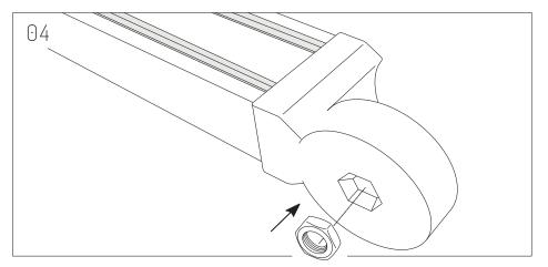
Insert Hex Nut on each Beam Bracket.
