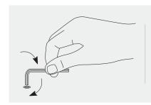
If this bolt does not drop into the joint use the Allen key to screw it all the way in so that it creates its own thread.
