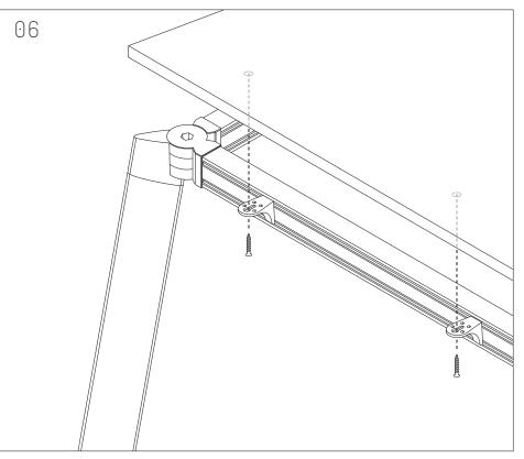
Directly screw into table tops, using L-Bracket screws through each L-Bracket.
