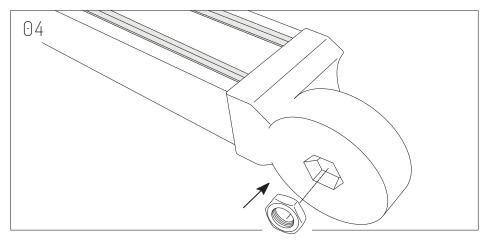
Insert Hex Nut on each Beam Bracket.
