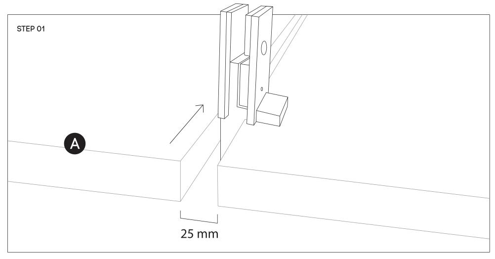
Please leave 25mm gap between table tops (A) so we can install pincer clamp brackets between the two table tops. Pincer brackets can be installed around 250mm-300mm from the end of the screen (or can be any desired distance).
