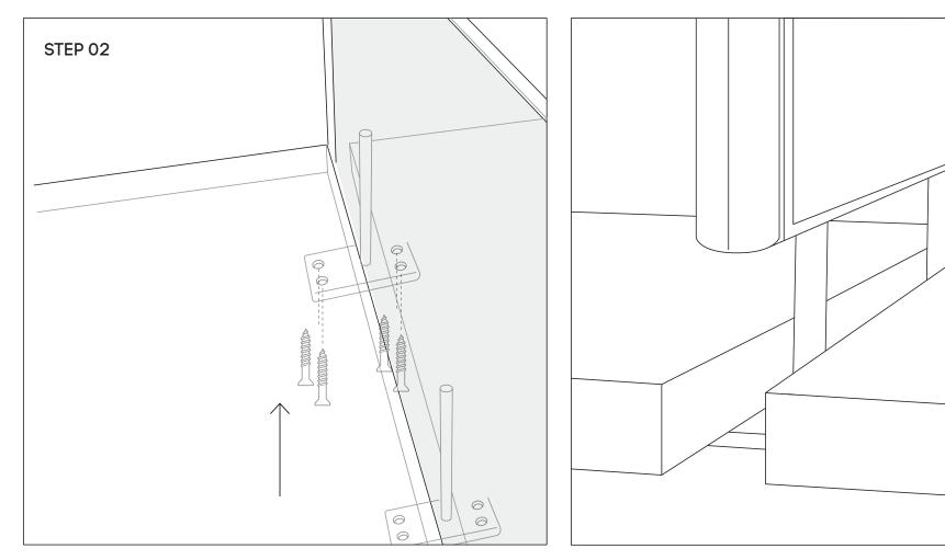
Second person to drill 4 holes into the brackets holes with provided wood screws into the underneath desktop. Please check the position of the rod brackets and bracket holes again before drilling the screws all the way through. Please tighten all the wood screws.
