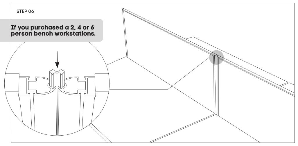
Using an Allen key remove top 2 caps from screens uprights. The two partitions should be next to each other. Please slide the 2 way connector rod - down between the two screen uprights.
