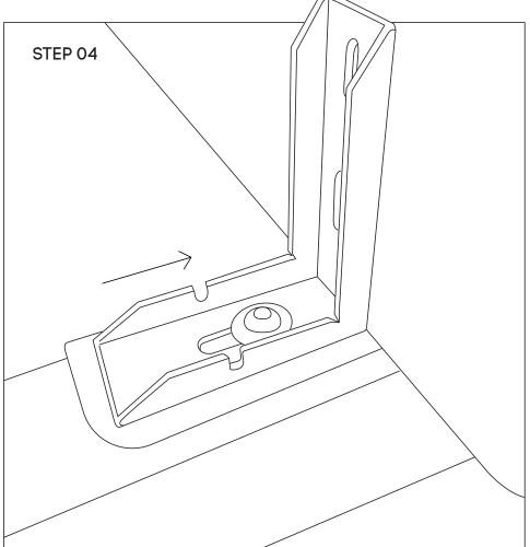
Step 3: Once the L-shape brackets are assembled, please place the screen in between the two L-Shape brackets.
