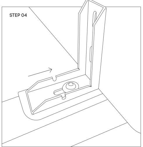
Step 3: Once the L-shape brackets are assembled, please place the Echo panel screen in between the two L-Shape brackets.
