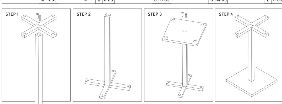
Note: To achieve the best results, we strongly recommend using an impact drill gun together with thread locking all screws.
