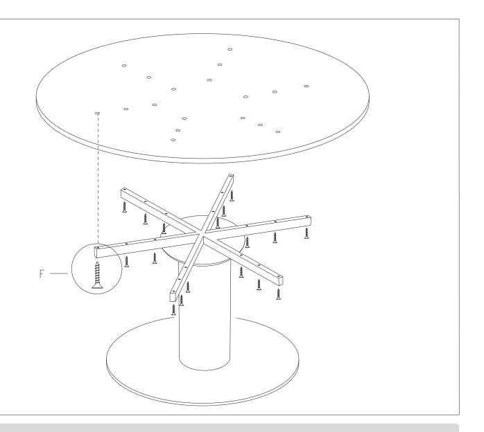
Note: To achieve the best results, we strongly recommend using an impact drill gun together with thread locking all screws.
