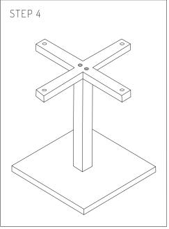
Note: To achieve the best results, we strongly recommend using an impact drill gun together with thread locking all screws.
