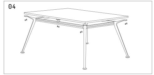
Ensure the worksurface is centered over the frame. Fully tighten all M5x20mm self tapping screws through each leg and rail space bracket into the worksurface.
