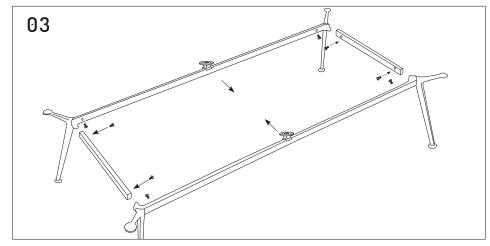
Securely connect legs to rails lenghts using the shorter M8x20mm dome head bolts.
