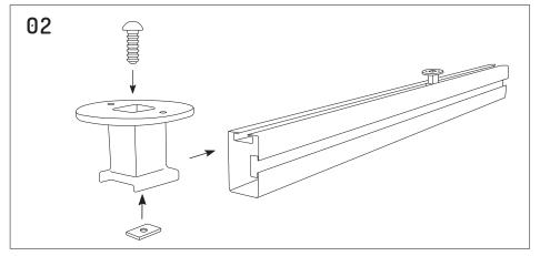
Loosely connect the longer M8x20mm dome head bolt and slot nut through the rail spacer bracket. Slide onto required rails and fully tighten in place.
