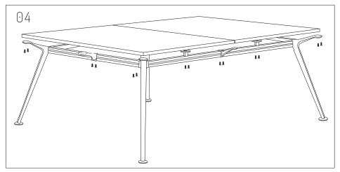
Ensure the worksurface is centered over the frame. Fully tighten all M5x20mm self tapping screws through each leg and support bracket into the worksurface.
