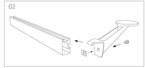
Loosely connect the shorter M8x12mm dome head bolt and slot nut through the metal rail spacer bracket. Slide onto 620mm rails.
