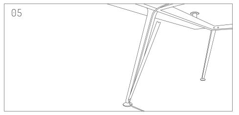
Conceal any power cable using the magnetic leg cable covers.
