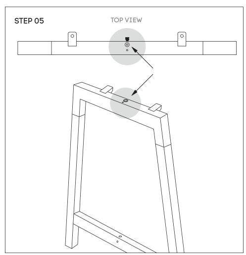
Attach Upper Beams **(E)** to legs using nut insert. See point attached
