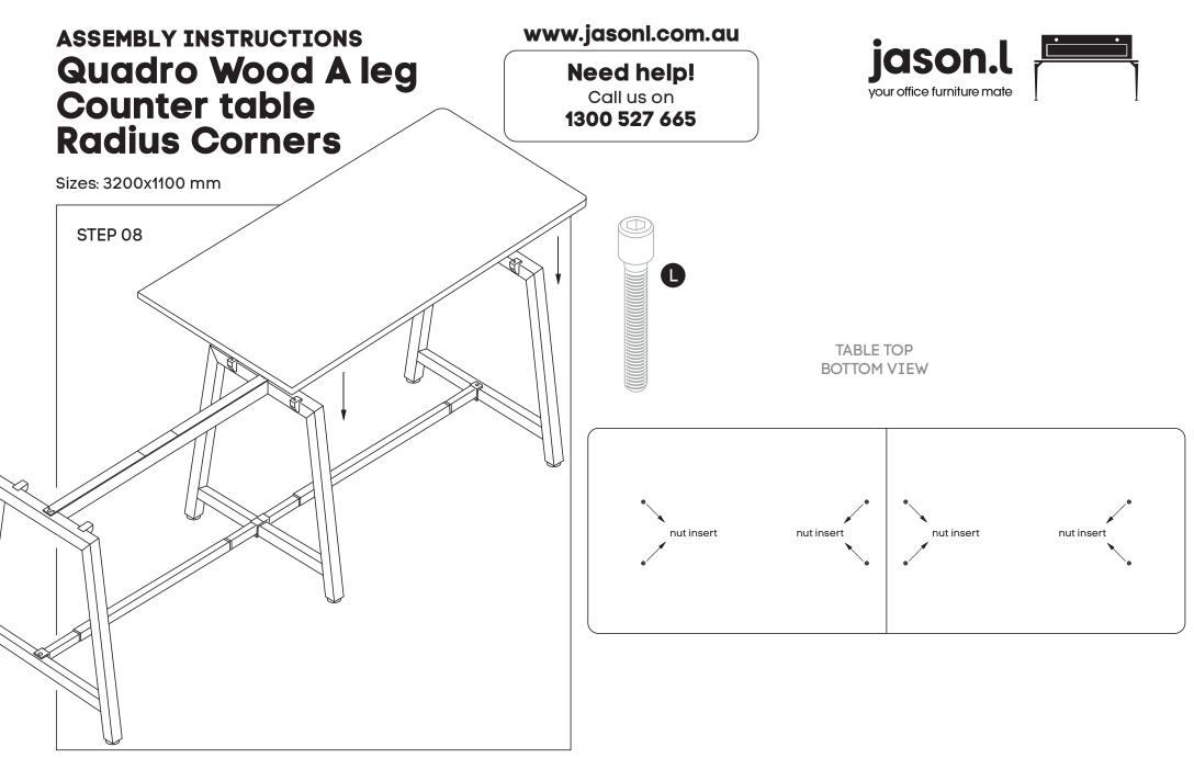
Place desktops ontop of frame. Nut inserts in top will align with plastic joiner brackets using M6x30MM **(L)** sockets attached top to frame.
