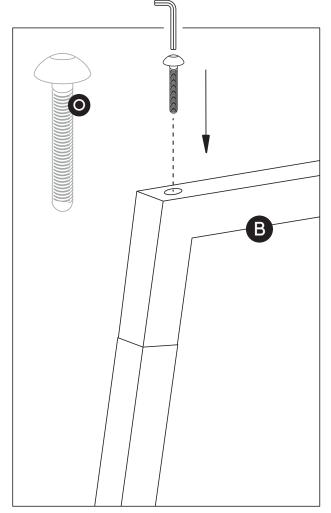
Insert the Leg wood add on **(C)** into the Leg Quadro A (Half leg) **(B)**. Using Allen Key provided, attach mushroom head screw **(O)** for all legs.
