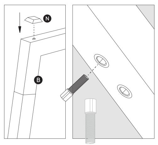
Now use corner pads **(N)**to cover the holes where just inserted the head screw sockets.
