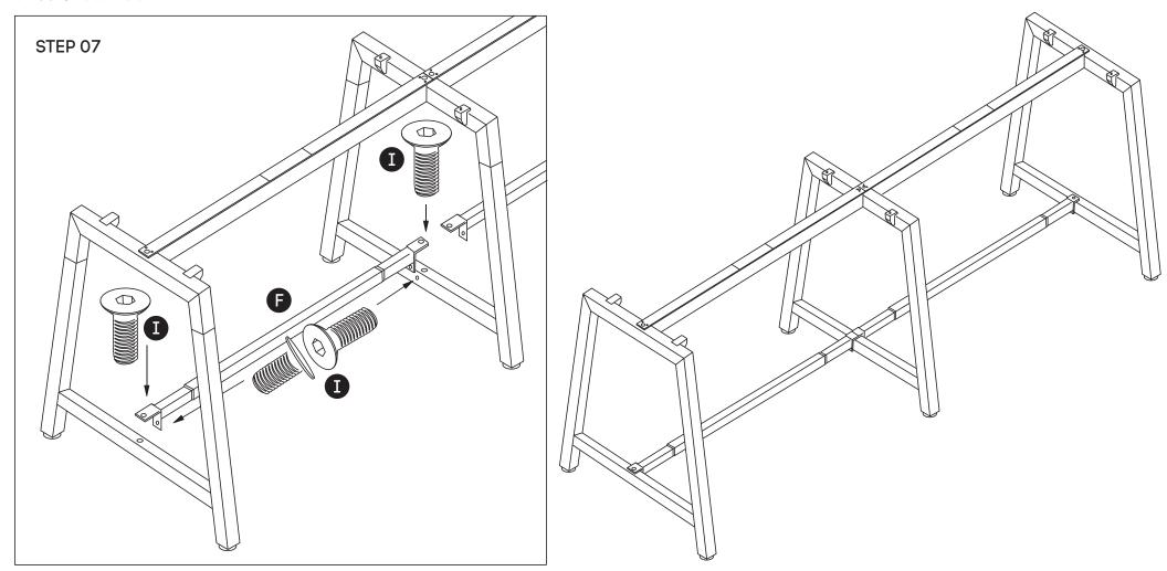
Frame looks like this. Using Allen Key. Tighen Sockets (I) on the Lower Beams (F) using Allen Key (O). Insert plastic spacers to improve regidity. Attach two Sockets (I) to the side of each lower side beams (as shown in the picture).
