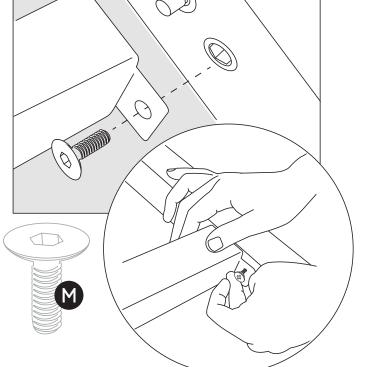
Now insert the Leg bottom beam (D) into the Leg wood add on (C), using Pins (M) provided. Attach on each leg.
