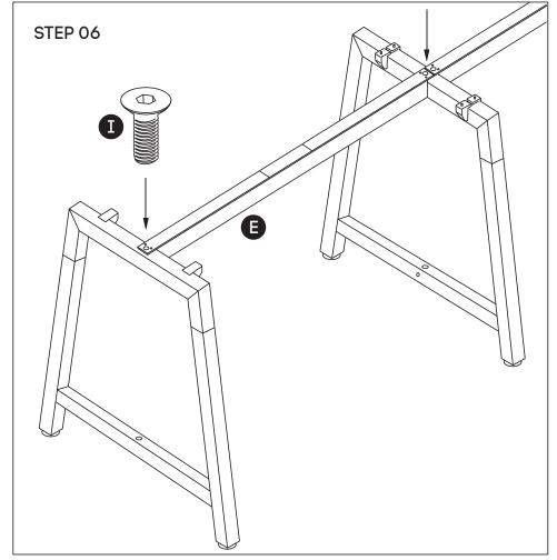
Frame looks like this. Using Allen Key, attach Upper Beams **(E)** with Sockets **(I)**.
