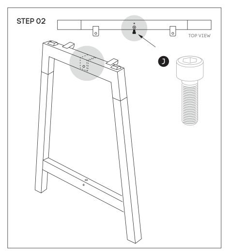
Using Allen Key provided, attach M8x20MM Socket head (J)-screw socket half way into leg for all legs
