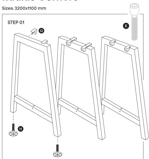
Using Allen Key provided, attach 2 plastic brackets **(G)** per exterior leg, and 4 plastic brackets for the shared leg (as per picture above) using M6x20MM **(K)** Socket head screw. Screw the feets **(H)** to the bottom of each Leg wood add on **(C)**.
