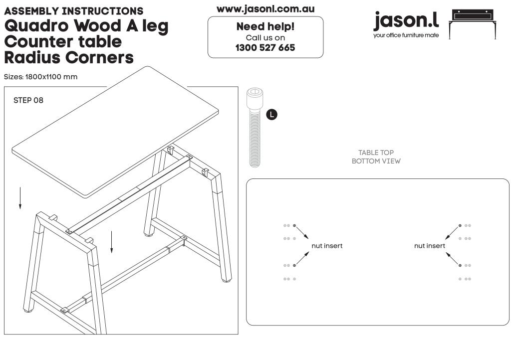
Place desktop ontop of frame. Nut inserts in top will align with plastic joiner brackets using M6x30MM **(L)** sockets attached top to frame.
