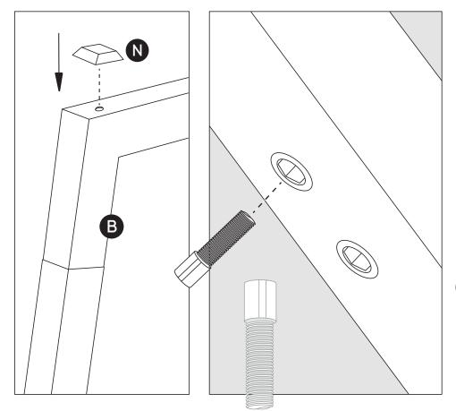
Now use corner pads **(N)** to cover the holes where just inserted the head screw sockets. You will notice two holes in each Leg wood add on **(C)**. Insert a Pin into the top hole of each leg, as shown in the illustration. Now insert the Leg bottom beam (D) into the Leg wood add on (C), using Pins (M) provided. Attach on each leg.
