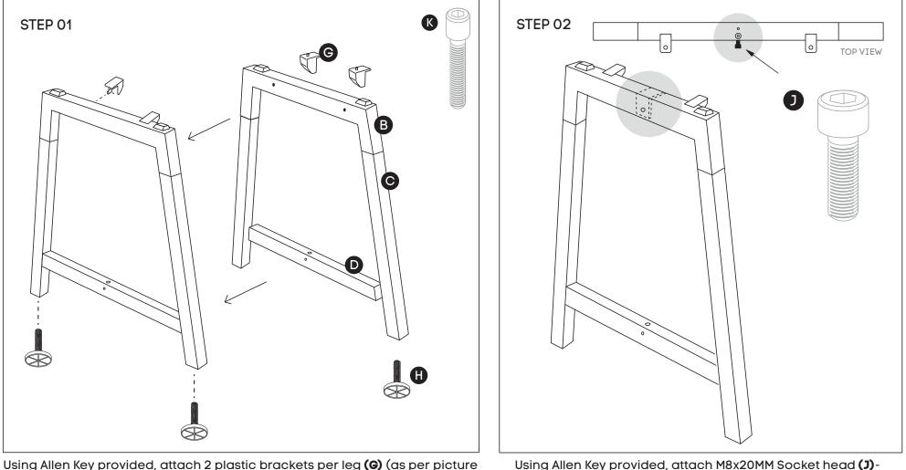
Using Allen Key provided, attach 2 plastic brackets per leg (G) (as per picture above) using M6x20MM (K) Socket head screw. Screw the feets (H) to the bottom of each Leg wood add on (C).
