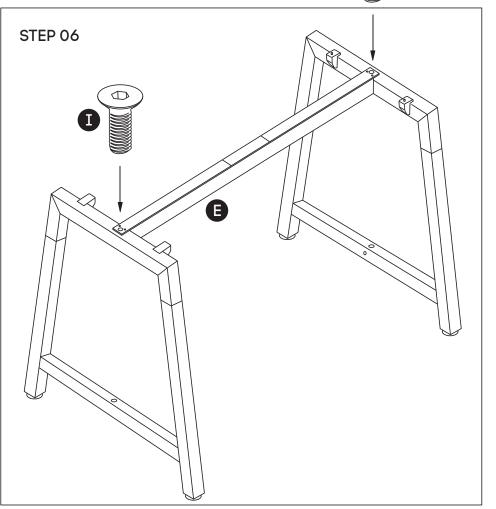
Frame looks like this. Using Allen Key, attach Upper Beam **(E)** with Sockets **(I)**.
