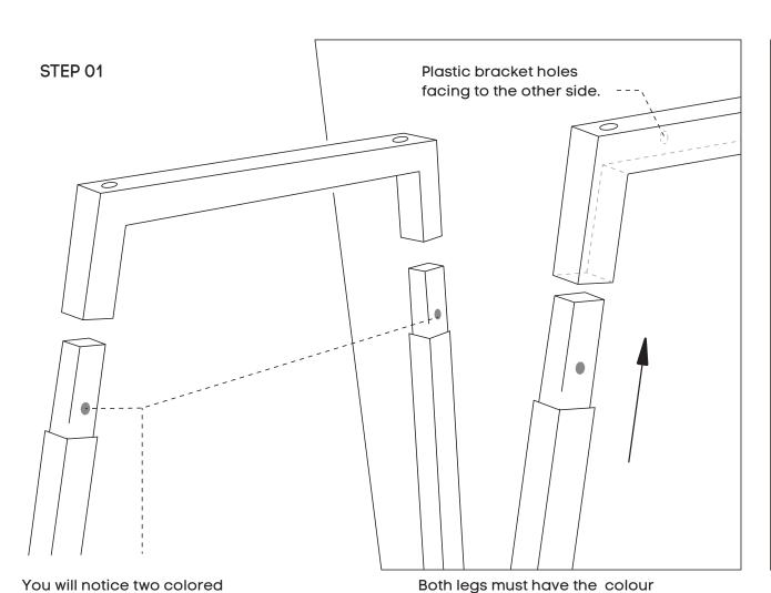
Insert the bottom of the legs as shown in the illustration. Using Allen Key provided, attach Mushroom Head Screw (J) - for all legs.
