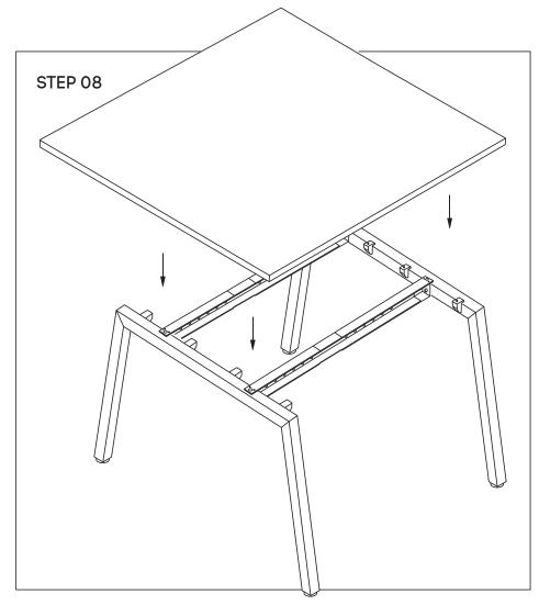
Place desktop on top of frame. Wood Screws to be drilled into the underneath Top.
