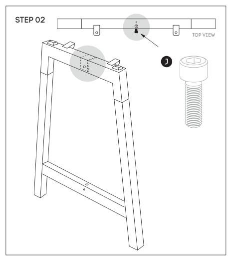
Using Allen Key provided, attach M8x20MM Socket head (J)-screw socket half way into leg for both legs
