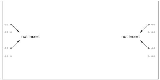
Place desktop ontop of frame. Nut inserts in top will align with plastic joiner brackets using M6x30MM **(L)** sockets attached top to frame.
