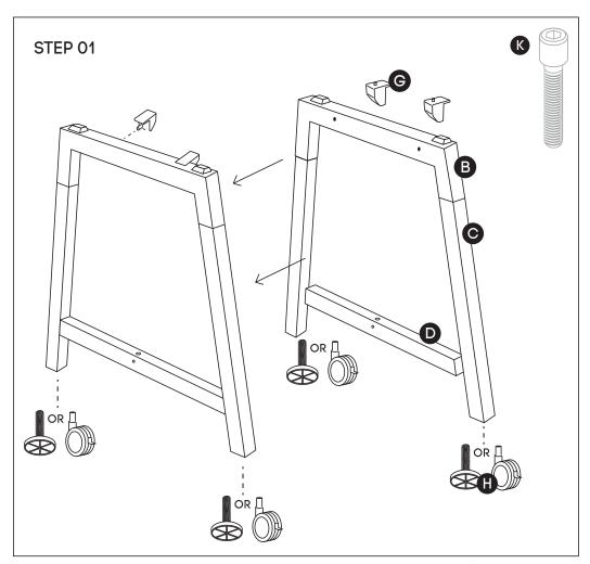
Using Allen Key provided, attach 2 plastic brackets per leg (G) (as per picture above) using M6x20MM (K) Socket head screw. Screw the feets or wheels (if you purchase with wheels option) (H) to the bottom of each Leg wood add on (C).
