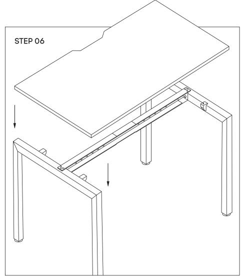
Place desktop on top of frame - with cutout at the back of the desk. Wood Screws to be drilled into the underneath Top.
